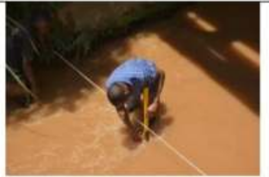
(j) Flow measurement using float (top width, length, time, depths of each interval)
