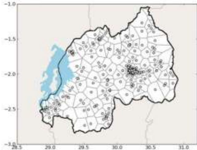
Figure 1. Map of Rwandan cell phone towers, January 2008. The median area covered each tower is roughly 70km 2 . Blumenstock 20
